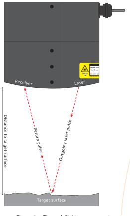
Figure 1:: Time-of-flight measurement
