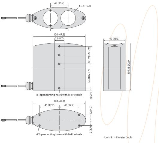
Figure 3:: Dimension drawings of the SF00
