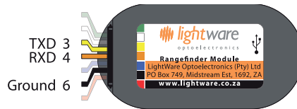
Figure 7 :: Serial interface connections
